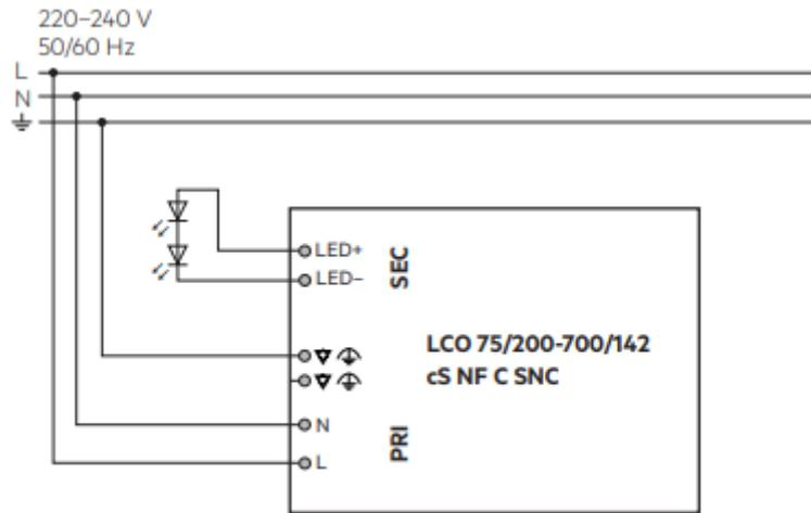
Both earth terminals have the same function and can be used interchangeably. (Through wiring not supported)
